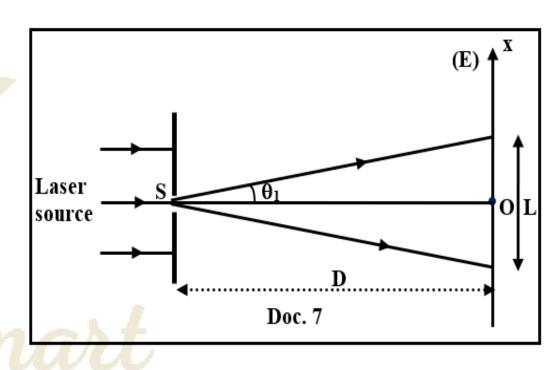
The screen (E) is placed parallel to the plane of the slits at a distance D = 2m. A laser source illuminates the slit by a monochromatic light of wavelength  $\lambda = 600nm$  in air, under normal incidence.
